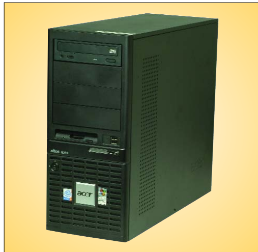
Acer Altos G310; based on a i875P chipset
